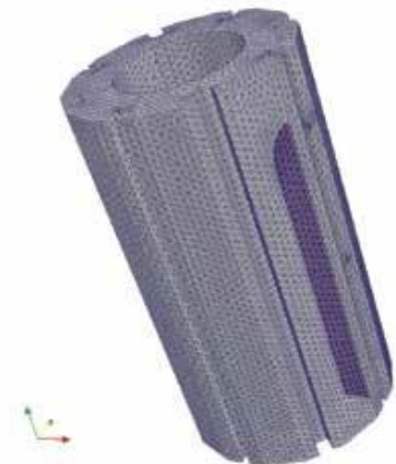
Cracked graphite moderator
