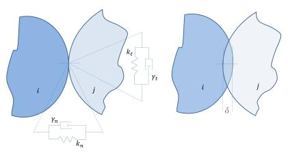
Spring displacement is given by body overlap,  $\delta$ , hence 'soft' body. This translates into a **penalty method**, solved with the same explicit schemes as the SPH equations.
