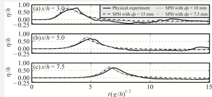
Convergence at  $x/h = 5.0$  and  $7.5$ , unclear at  $x/h = 3.0$  (non-linearities, multi-phase effects due to slide impact);  $dp = 10 \text{ mm}$  seems an appropriate compromise between simulation time and accuracy
