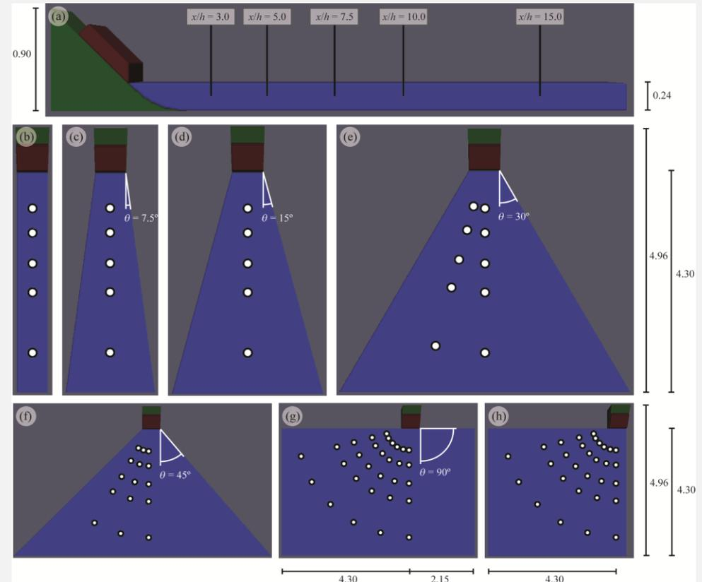
All geometries: (a,b) side and plane view of 2D case, (c) basin side angle  $\theta = 7.5^\circ$ , (d)  $15^\circ$ , (e)  $30^\circ$ , (f)  $45^\circ$ , (g)  $90^\circ$  (3D) and (h) 3D corner case 3Dc
